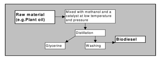
The raw oil is reacted with an excess of alcohol (often methanol or ethanol) in the presence of a catalyst (often potassium or sodium hydroxide). The products of this reaction are crude biodiesel and crude glycerine, with an excess alcohol, which is recovered and re-used.
